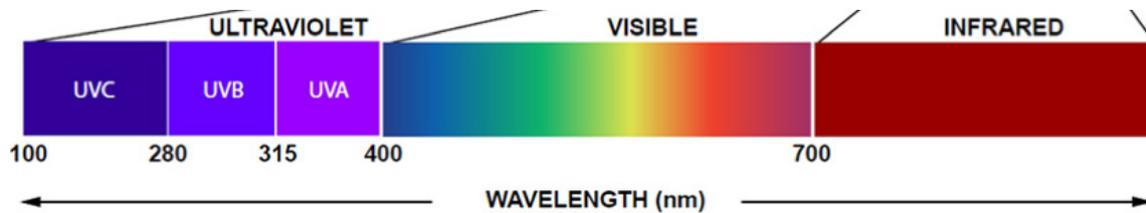
For many years, UVC light has been used in industry and in hospitals for disinfection. UVC light has a wavelength of 253.7 nm and is, therefore, invisible to the human eye. Many UVC light sources also emit other wavelengths, and therefore, you often see the light as blue or violet, but it is not the UVC light itself you can see.
